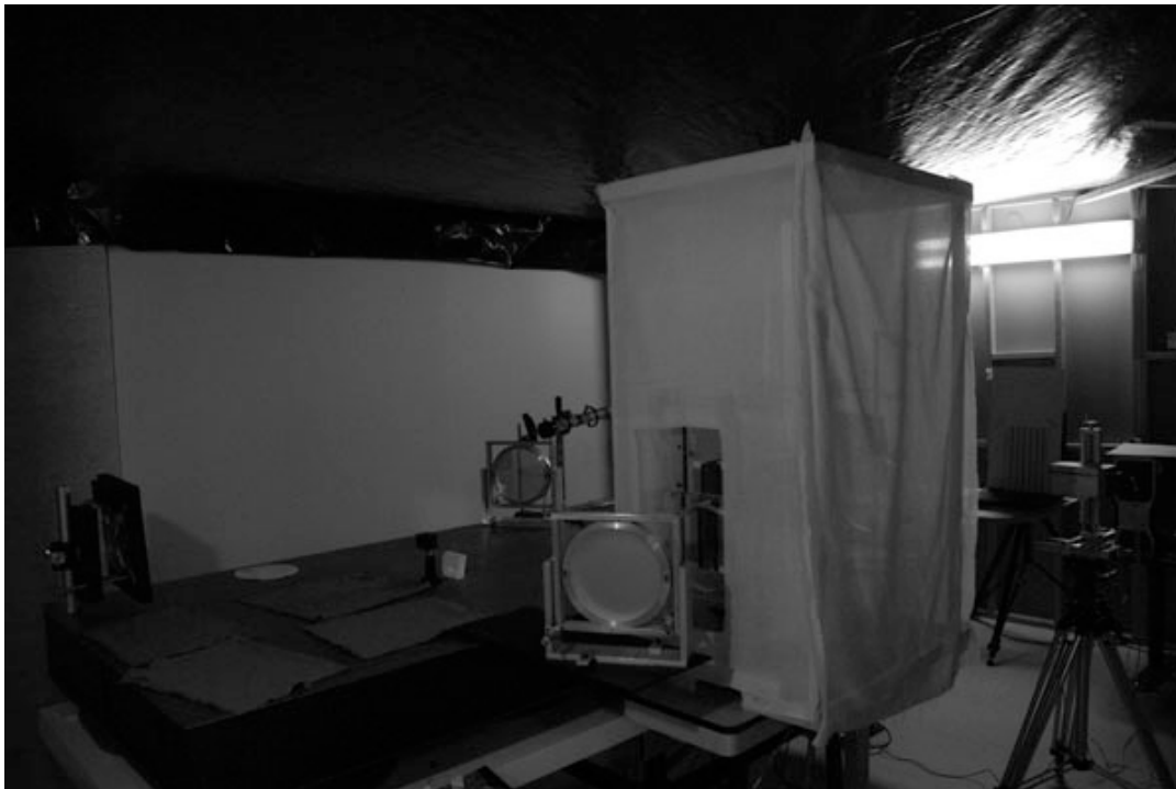
Figure 2.7: Photograph of the experimental model with the “eddy tent” in the interferometer.
