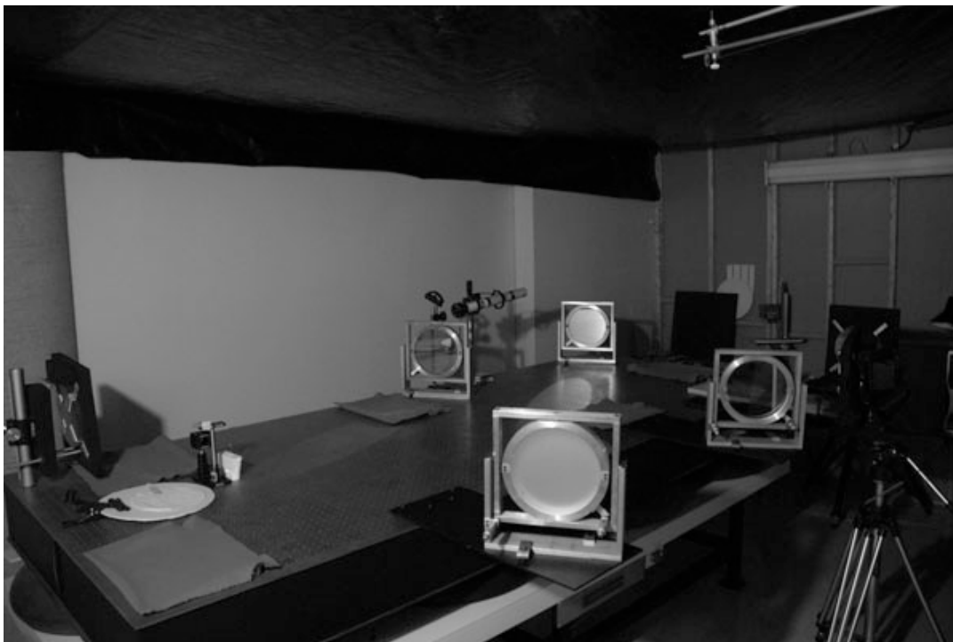
Figure 2.2: Photograph of the Mach-Zehnder interferometer.
